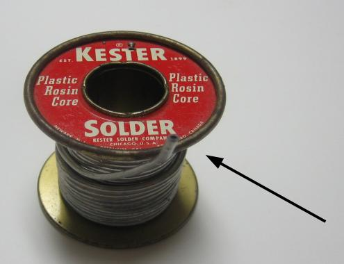
Look closely and you can see the hollow core of the solder, which is filled with flux.
