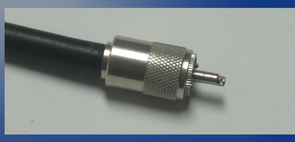
The RG-8X cable is smaller and requires an adaptor to fill the space between the cable and the connector. The adapter comes in two sizes so make sure you have the correct adapter to fit your size cable.
