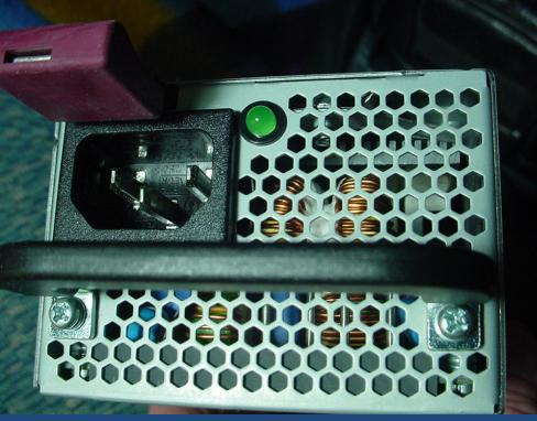
The front has the AC cord input, the power ON indicator light, and a handle. The front is perforated for cooling. These power supplies were used in "server farms". They can be hot swapped and provide current sharing in their intended environment. Lucky for Ham operators technology changes quickly and we become the benefactors of this technology on the surplus market.
