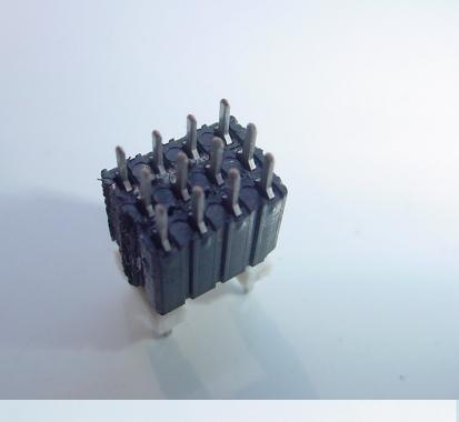
What we are now going to do is take the header we constructed and add on a 330 ohm resistor and a couple of wires to "program" the power supply to our desired use. This configuration gives us 13.6 v @47a. Why use a 330 ohm resistor? Well I did not have the size to make it 13.8v in my tray but I have several 330 ohm so that was the deciding factor. A 1K variable resistor can be substituted for the 330 ohm and you can vary the supply from 12v to 13.82v.
